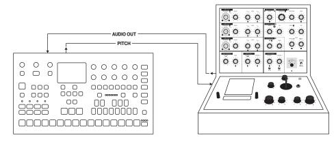
The CV/Gate outputs and the external inputs allow an external oscillator to be used with the internal Analog Four MKII oscillators. Use this trick when you want a different (perhaps old, quirky and unpredictable yet charming) oscillator to provide the fundamental tone but still want the control and modulation power of the Analog Four MKII.
