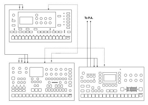
The Analog Four MKII thrives with other Elektron gear. In this example, it is used with an Octatrack and a Monomachine. The Monomachine main output is connected to the Analog Four MKII inputs. The Analog Four MKII main output is connected to one of the input pairs of the Octatrack. The main outputs of the Octatrack go to the PA. The Monomachine and Analog Four MKII are MIDI slaved to the Octatrack.
