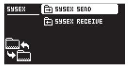
When receiving or sending SysEx data, the MIDI ports or the USB port of the Analog Four MKII should be connected to the external sending/receiving device.
