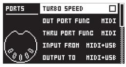
**TURBO SPEED** selects the multiplier of the MIDI transfer rate that will be used when the Analog Four MKII MIDI IN/OUT ports are connected to the MIDI OUT/IN ports of a turbo protocol compatible device. The [LEFT]/[RIGHT] arrow keys are used to select the multiplier. If AUTO is chosen, press [YES] to start the turbo speed negotiation.
