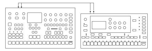
Thanks to the neighbor routing, all the filters of the Analog Four MKII can be used for providing an immense mono filter bank consisting of 8 filters plus 4 overdrive circuits. The setup can be either serial or parallel. It can, of course, be set up for stereo filtering as well. In this scenario, 4 filters are available for the left and right channels.
