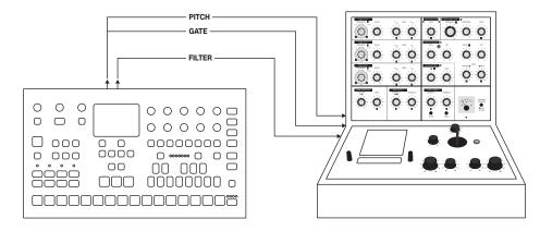
The CV/Gate track of the Analog Four MKII is made for controlling external, CV/Gate equipped, analog gear. In this scenario, a vintage analog synthesizer is controlled by the Analog Four MKII. The pitch and filter cutoff will be controlled.
