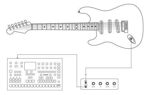
In this setup example, the Analog Four MKII is used for processing the sound output from an electric guitar. The first, most basic method uses the FX track to turn the Analog Four MKII into an effects box sporting the Wideshift Chorus, Saturator Delay, and Supervoid Reverb effects. The second, more elaborate method routes the sound through Track 1 and allows all the sound-shaping possibilities offered by the FILTERS, AMP, ENV and LFO.
