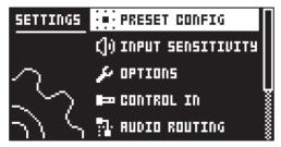
Scroll through the list of settings by using the *NAVIGATION* knob. Open a highlighted menu by pressing the *NAVIGATION* knob or **[YES]**. To change the settings in the menus, first press, and then turn the *NAVIGATION* knob.
