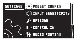
Scroll through the list of settings by using the *NAVIGATION* knob. Open a highlighted menu by pressing the *NAVIGATION* knob or [YES]. To change the settings in the menus, first press, and then turn the *NAVIGATION* knob. For more information, please see "6. THE SETTINGS MENU" on page 17.
