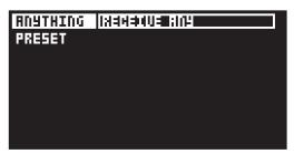
The column to the left selects what will be received. Use the *NAVIGATION* knob to navigate in the column. The SysEx data receive alternatives located in the column to the right will change depending on the selection made in the left column. Press [YES] to access this column. Use the *NAVIGATION* knob to select what will be received. Press [YES] to initiate the SysEx receive procedure. The Analog Heat +FX starts listening to incoming data. Press [NO] to stop listening.
