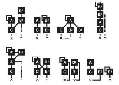
The lines going to X and Y indicate the output from a carrier. There are two different ways a carrier output is sent to the X/Y outputs: 1. Its amplitude is unaffected by the operator envelope (dotted line). 2. Its amplitude is affected by the operator envelope (filled line). The sound from the X/Y outputs is then routed via the overdrive to the filters.
