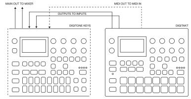
Digitone Keys works very well together with the Digitakt, and you can, for example, route the audio from the Digitakt through the Digitone Keys and sync the tempo of the sequencers.
