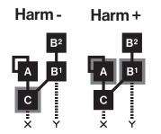
When changing harmonics, intermediate values interpolates between the current and the next harmonic. This interpolation works much like in wavetable synthesis, sweeping between the harmonics, smoothly transitioning from one timbre to another. For more information, please see "11.3.5 HARM" on page 49. The harmonic series for the operators looks like this:
