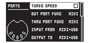
**TURBO SPEED** press **[YES]** to start the turbo speed negotiation. The device chooses the optimal speed automatically. Please note that you must use a MIDI interface that supports the Turbo-MIDI protocol.
