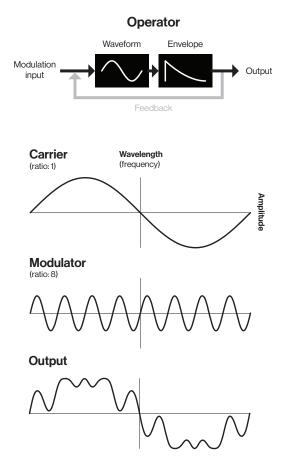
In some instances, an operator can be both carrier and modulator. This means that it outputs its result as a tone while also using it to modulate another operator. We have divided the operators into three groups: **C**, **A**, and **B** (B1 and B2) to lessen the complexity and make the Digitone Keys easier to use. Since group **B** consist of two operators, the parameter controls for **B** are macro mapped to both operators.
