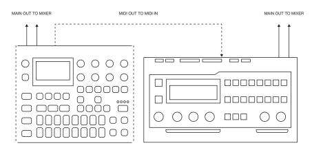
Digitone Keys has extensive MIDI sequencing capabilities and can use its MIDI tracks to control other MIDIequipped synthesizers.
