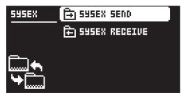
When receiving or sending SysEx data, the MIDI ports or the USB port of the Digitone Keys should be connected to the external sending/receiving device.
