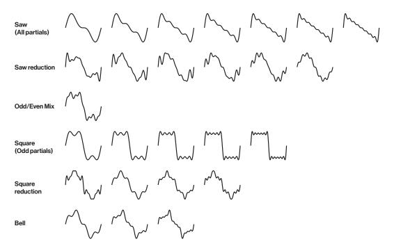
The Digitone Keys uses a form of additive synthesis to create the harmonic series for the **HARM** parameter. Additive synthesis is one of the oldest forms of electronic sound generation. It is a quite simple form of synthesis but still very powerful. The basic principle is to add multiple sine waves together to form complex timbres. Each sine wave is called a partial. By attenuating each partial, the timbre changes its harmonic content, resulting in different waveforms.
