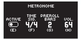
ACTIVE activates/deactivates the metronome. You can also press [FUNC] + [PTN] and hold for a second to toggle the metronome on and off when you are not in the METRONOME menu.
