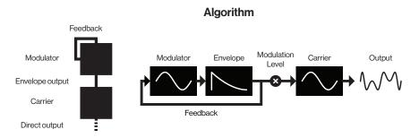
Pictured above is a 2 operator algorithm, which is FM synthesis in its most basic form. The Digitone Keys has four operators available which can be routed in many different ways. Different algorithms dramatically changes the characteristics of the output - for example stacking four operators can lead to very complex timbres.
