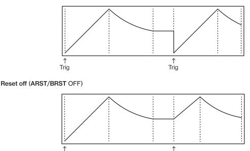
The **LEVEL** parameters on the SYN2 page controls the amount of modulation from the A and B operators. For more information, please see "11.5.8 LEV B" on page 51. The **LEVEL** parameter for B is macro mapped to both operator B1 and B2 and control their modulation amount as per this graph:
