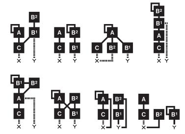
The lines going to X and Y indicate the output from a carrier. There are two different ways a carrier output is sent to the X/Y outputs: 1. Its amplitude is unaffected by the operator envelope (dotted line). 2. Its amplitude is affected by the operator envelope (filled line). The sound from the X/Y outputs is then routed via the overdrive to the filters.
