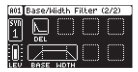
The base-width filter is basically a Highpass filter and a Lowpass filter connected in series. The filters **BASE** and **WIDTH** parameters define the base-width filters frequency range.
