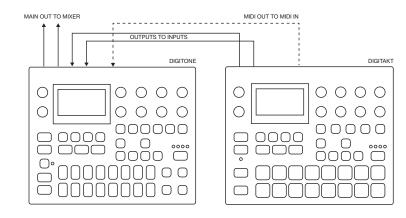
Digitone works very well together with the Digitakt, and you can, for example, route the audio from the Digitakt through the Digitone and sync the tempo of the sequencers.
