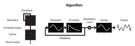
Pictured above is a 2 operator algorithm, which is FM synthesis in its most basic form. The Digitone has four operators available which can be routed in many different ways. Different algorithms dramatically changes the characteristics of the output - for example stacking four operators can lead to very complex timbres.
