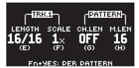
The TRACK column sets the step length and scale of the track. The settings only affects the active track. Press the **[TRK]** keys to select the track whose scale settings you wish to edit.
