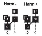
When changing harmonics, intermediate values interpolates between the current and the next harmonic. This interpolation works much like in wavetable synthesis, sweeping between the harmonics, smoothly transitioning from one timbre to another. For more information, please see "11.3.5 HARM" on page 47. The harmonic series for the operators looks like this:
