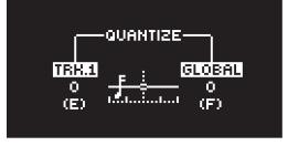
**TRK.** affects the trigs of the active track in real time. The higher the quantize value, the more the trigs are quantized. Press **[T1–4]** key to select what track to quantize. (0–127)
