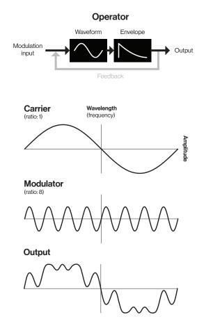
In some instances, an operator can be both carrier and modulator. This means that it outputs its result as a tone while also using it to modulate another operator. We have divided the operators into three groups: **C**, **A**, and **B** (B1 and B2) to lessen the complexity and make the Digitone easier to use. Since group **B** consist of two operators, the parameter controls for **B** are macro mapped to both operators.
