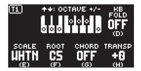
**SCALE** sets the tracks scale. This is done by limiting which keys are playable on the Digitone keyboard and from external MIDI devices that sends on the Digitone's AUTO channel. For a list of all selectable keyboard scales, please see "APPENDIX D: KEYBOARD SCALES" on page 100.
