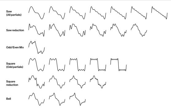
The Digitone uses a form of additive synthesis to create the harmonic series for the **HARM** parameter. Additive synthesis is one of the oldest forms of electronic sound generation. It is a quite simple form of synthesis but still very powerful. The basic principle is to add multiple sine waves together to form complex timbres. Each sine wave is called a partial. By attenuating each partial, the timbre changes its harmonic content, resulting in different waveforms.
