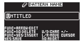
The [LEFT] and [RIGHT] arrow keys are used to navigate between the characters. Turning the LEVEL/ DATA knob or pressing the [UP] or [DOWN] arrow keys selects the characters. [FUNC] + [NO] erases letters. [FUNC] + [YES] inserts space.
