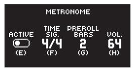
ACTIVE activates/deactivates the metronome. You can also press [FUNC] + [PTN] and hold for a second to toggle the metronome on and off when you are not in the METRONOME menu.
