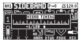
MICRO TIMING Press [LEFT]/[RIGHT] keys to adjust the time offset.
