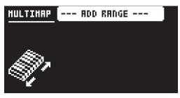
**RANGES** are the basic building blocks of the multi map. They define what function that is assigned to each key or key range. A multi map can contain up to 128 ranges. The ranges can be set within the note interval CO–G10 If no ranges exist, select ADD RANGE.
