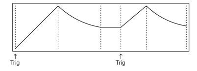
The **LEVEL** parameters on the SYN2 page controls the amount of modulation from the A and B operators. For more information, please see "11.5.8 LEV B" on page 49. The **LEVEL** parameter for B is macro mapped to both operator B1 and B2 and control their modulation amount as per this graph:
