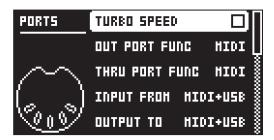
**TURBO SPEED** press **[YES]** to start the turbo speed negotiation. The device chooses the optimal speed automatically. Please note that you must use a MIDI interface that supports the Turbo-MIDI protocol.
