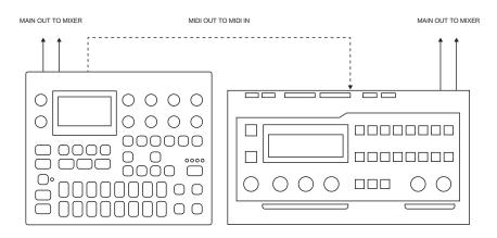
Digitone has extensive MIDI sequencing capabilities and can use its MIDI tracks to control other MIDIequipped synthesizers.
